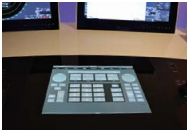
Virtual ECDIS / Chart Radar keyboard control on the touch screen monitors
