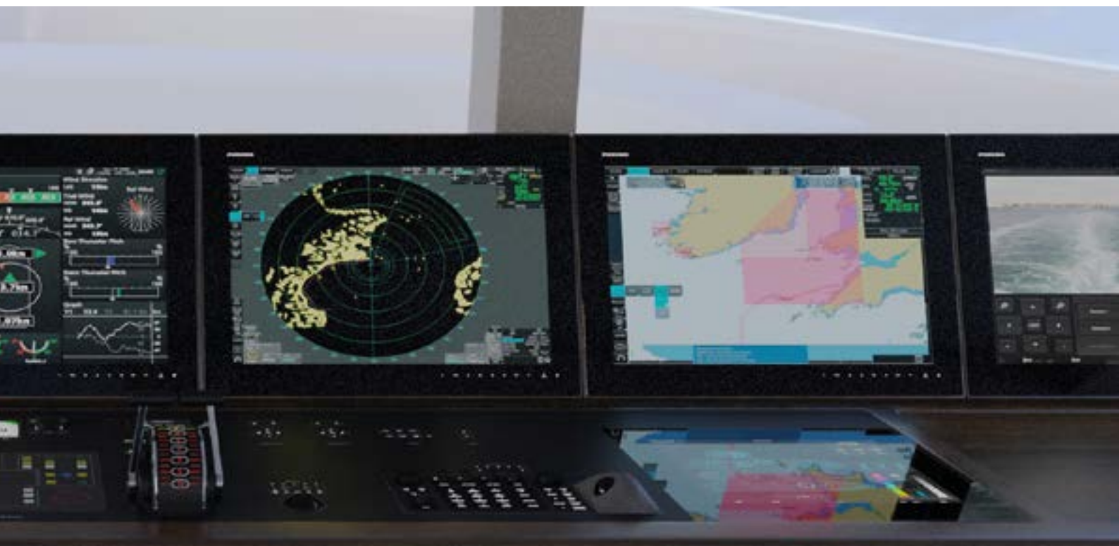
Original Chart Radar / ECDIS keyboards fully integrated in the helm panel
