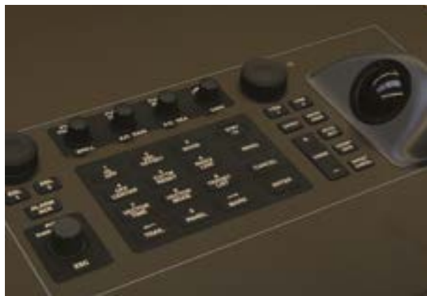
Original Chart Radar / ECDIS keyboards fully integrated in the helm panel
